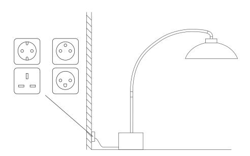
NOTE: The DOME will be delivered with a supply cord of 2 m 90.
